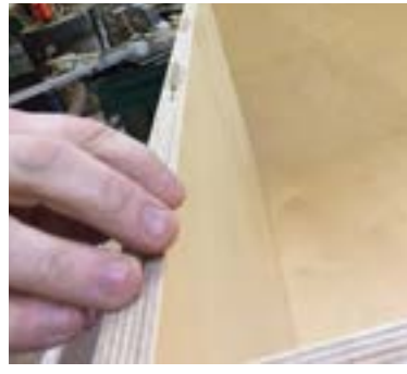
Biscuit jointing birch plywood cabinets
